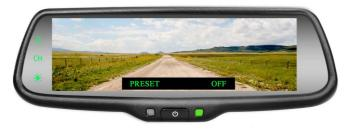
The reversing mode is the top priority, then all touch panel is ineffective. The video cannot be switched until the parking mode is ended. But the manual button is accessible. Short press is to adjust the brightness of the monitor, long press to turn off the screen.
